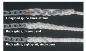
Square line, also known as eight-stranded plaited rope, is a single-core, extremely flexible and soft rope that resists kinking and coils neatly into the anchor locker with little or no tending. Because of its flexibility, the same length of eight-stranded plaited takes up less stowage space than the same length of three-strand. If you are installing a new windlass and need a new line and chain, go the extra
