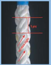
Learn right and left. Eight plait, sometimes called square line, has four distinct surfaces or sides. When you turn the rope 90 degrees, its top strands appear to rotate as a pair to the right; turn it another 90 degrees, and the top strands or pairs will rotate to the left. On each of the four sides there is a pair of strands rotating together in the same direction. Study the rope before you begin and learn the left and the right.
