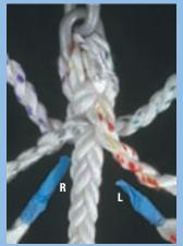
Confused yet? At this point you have done four tucks. Examine your work. Are both right pairs running from right to left under a left rotating pair? Do they have a partner weave under them running in the same direction? Are both left pairs running from left to right under a right rotating pair? Do they have a partner weave running in the same direction under them? If you answered yes to each question, good job.
