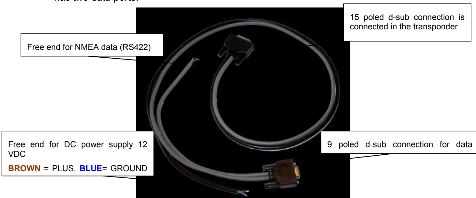
Figure 9 AIS-CTR X CARBON data and DC cables
