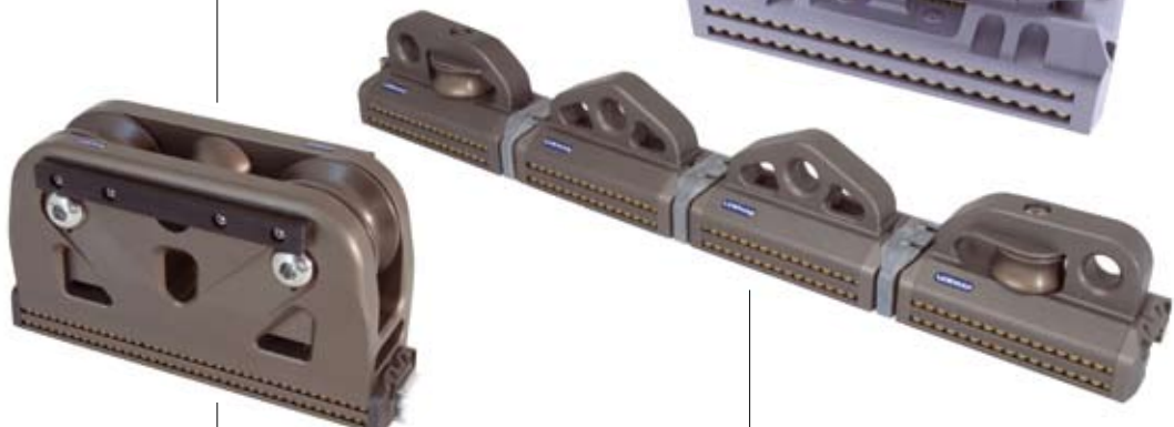
The Lewmar custom racing blocks feature PTFE impregnated main bearings with two rows of torlon side thrust balls making the block very efficient.
