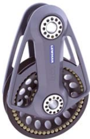
The Lewmar custom racing blocks feature PTFE impregnated main bearings with two rows of torlon side thrust balls making the block very efficient.
